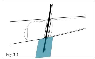
(f) Repeat Steps 3(a) - 3(e) for the RH rear door molding placing the front edge of the molding 5.5 mm from the door edge as shown (Fig. 3-3 and Fig. 3-4).
