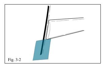
**NOTE:** Once the release liner is removed from the molding, the surface of the foam tape must not be touched.
